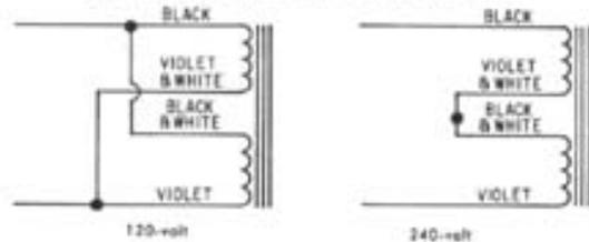
Stereo 70s supplied with power transformer PA-521 may be connected for either 120 volt or 240 volt AC operation as follows:
