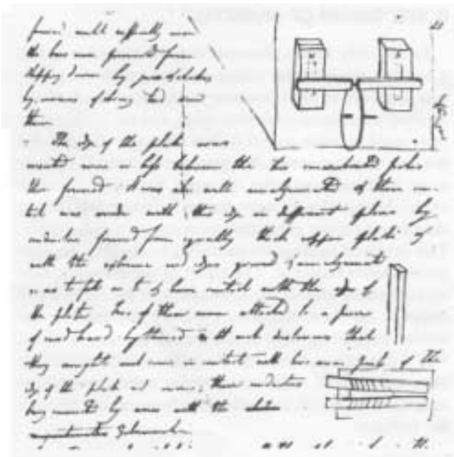
Fig. 3. Page from Faraday's diary showing sketch of first dynamo.
