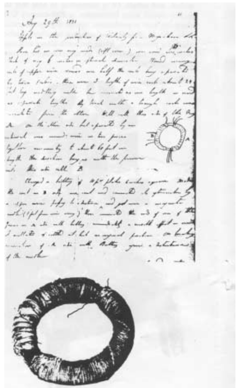
Fig. 2. Page from Faraday's diary describing experiment and showing his induction ring the first toroidal transformer.
