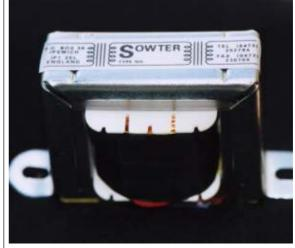
**APPLICATION** Designed to be driven from a cathode follower output stage via a coupling capacitor. Suitable for headphones with an impedance in the range 30 to 600 ohms.
