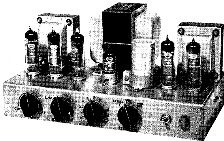
Prototype of Seven-watt Stereophonic Amplifier
