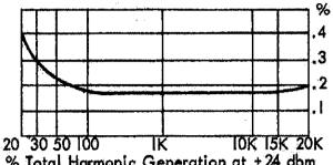
% Total Harmonic Generation at +24 dbm into rated load. Amp. strapped "high".
