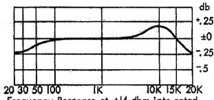
Frequency Response at +14 dbm into rated load. Source: Rated.
