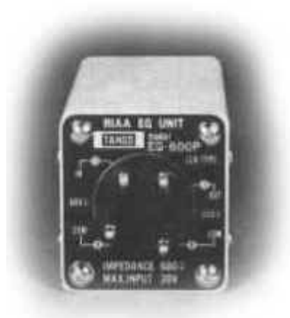
Fig. 7 The TANGO EQ-600P LCR Unit
