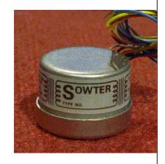
**APPLICATION** For use as a line input or in reverse mode for a low power output transformer for tube or solid-state amplifier. Ideal for use with a CD player or sound card to provide a balanced isolated line output. Centre tap on secondary so the transformer can be used as a phase splitter for use in a push-pull amplifier. Available with leads or for PCB mounting
