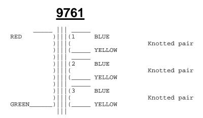
NOTE: Polarity is important on this transformer. Green and Yellow must be connected to ground. Red and Blue must be hot.
